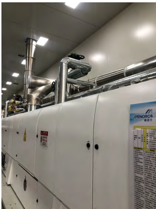
辊涂补伤线及配套排气筒
